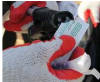
Application of petroleum jelly to spray gun
